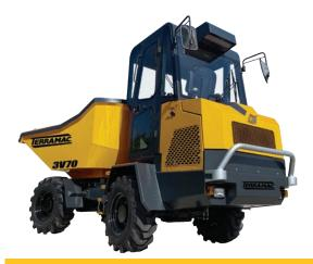
Frame Type: Articulated (3V70); Rigid (120TW) Bed Slewing Angle: 180°
