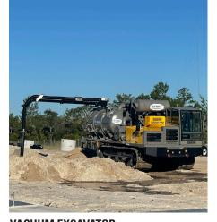
**VACUUM EXCAVATOR** Accelerates powerline repair by easily maneuvering over some of the most difficult jobsite conditions. Equipped with 5200 CFM, this unit quickly locates underground utility lines so new poles and lines can safely be set.
